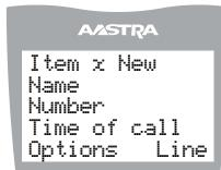
The above screen shows the item number, the name and number of the caller, and the time the call was received. Also shown are two soft keys — **Options** and **Line**. **Options** allow the user to save to directory or delete the record.
