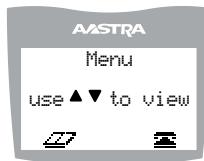
Navigation of the menu is performed using the down arrow (5 key) or the up arrow (4 key). Shortcut to the menu item can also be performed by pressing the corresponding menu item number. Two digits numbered items can be short-cutted by pressing the digits within a one second time span.
