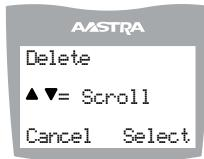
The user is prompted to confirm the delete action by pressing the **Delete** softkey.
