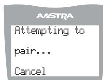
Upon success or failure of pairing, one of the following will be displayed on the handset and base, respectively:
