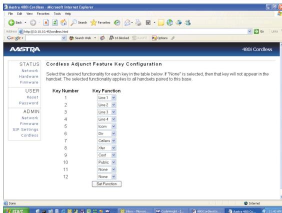
Once the functions are programmed, click on the **Set Function** button at the bottom of the page. This action will send the programming information to the phone and the key programming will be sent out to the cordless handsets. Any key programmed to "None" will not appear in the handset's list.
