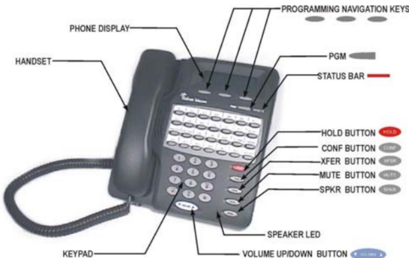
The *Emerald ICE* Standard Model Telephone features a speakerphone, 14 programmable Feature/DSS buttons (dual color LED), Headset Jack, 8 fixed feature keys (Mute, Speaker, Hold, Transfer, Conference, Feature, Volume Up, Volume Down), and one Status Bar type message waiting lamp.
