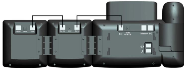
**Note:** Users can connect up to six modules. Connect the **Ext in** port of the previous module and the **Ext out** port of the next module with a connecting cord.
