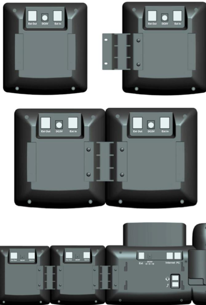
**Note:** The phone can support up to six expansion modules. If you use more than three expansion modules, you will need to connect an additional power adapter to any one of the expansion modules.
